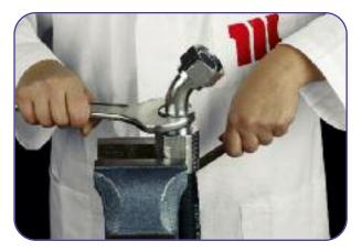
8 Insert the fitting into the hose. Press slightly and screw by hand turning clockwise the first threads. Then by using an appropriate spanner or a screwspanner on the hexagon, screw the fitting into the socket with a continuous and constant rotation motion and verify any absence of hose rotation inside the socket during the fitting screwing. Complete the screwing until the fitting reaches the bottom against the socket. Never overtighten. Assembling is now finished.
