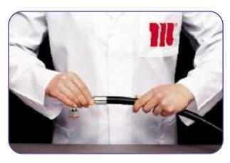
**5** Find the correct orientation and insert completely the fitting into the hose.
