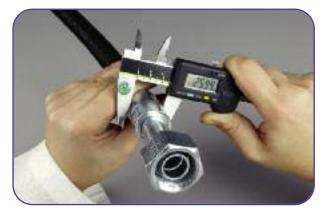
9 Inspect the crimping dimension using a calibrated vernier. Check the diameter at the centre of the ferrule following the values in table a.
