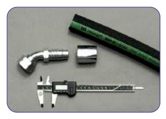
1 Check the dimensions of the components.
