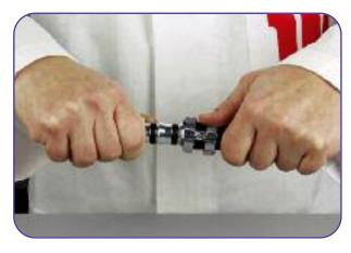
**6** Find the correct orientation and insert completely the fitting into the hose.
