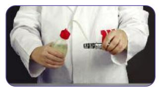
**5** Grease the end of the fitting joint with the same oil used in the air conditioning system.
