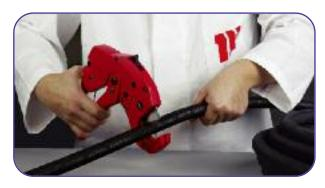
2 Cut the end of the hose in a perpendicular direction, using the manual cutter.
