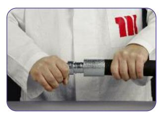
Find the correct orientation and insert completely the fitting into the hose.
