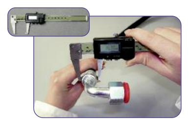
8 Inspect the crimping dimension using the proper calibrated vernier. Check the dimensions following the values in table c.
