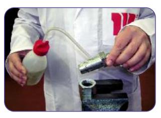
**7** Position the hose complete with socket i.e. by using a bench vise. Grease with a lot of oil the threading and the taper of the fitting as well as the inside of hose.
