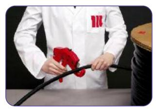
2 Cut the end of the hose in a perpendicular direction, using the manual cutter.
