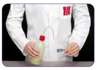
**4** Grease the end of the fitting joint with the same oil used in the air conditioning system.
