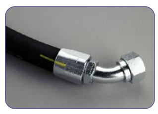
**9** You can leave a margin of max 3 mm between the hexagon of the fitting and the socket. Verify allignment.
