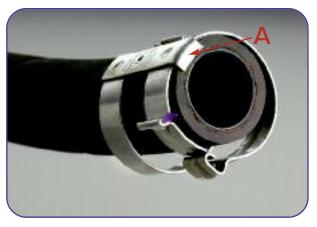
4 Place the double clamp on the flexible hose in such a way that the tooth of bar A comes contact with the end of the hose that has been cut.
