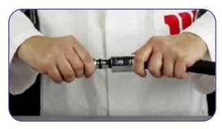
**6** Find the correct orientation and insert completely the fitting into the hose.
