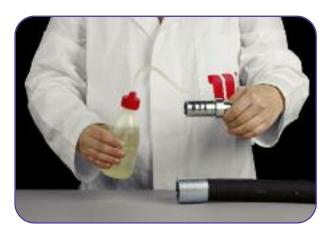
Grease the end of the fitting joint with the same oil used in the air conditioning system.
