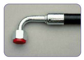
**6** Check the correct position of the hose through the proper hole in the ferrule.
