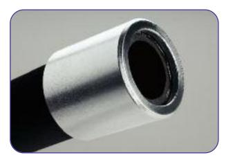
**5** Place the ferrule on the flexible hose so that the ferrule tooth touches the end of the cut hose.
