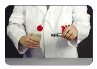
**5** Grease the end of the fitting joint with the same oil used in the air conditioning system.
