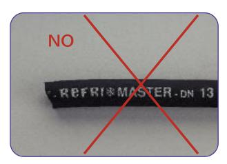
**3** Verify the end of the hose to be cut in a perpendicular direction.
