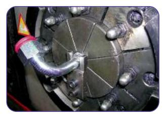
**7** Set up the criping machine selecting the die set that is closed to the dimension specified diameter. Place the fitting on the proper positioner to ensure that it is in the correct position (table c).
