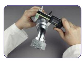
Inspect the crimping dimension using a calibrated vernier. Check the diameter at the centre of the ferrule following the values on the table b.
