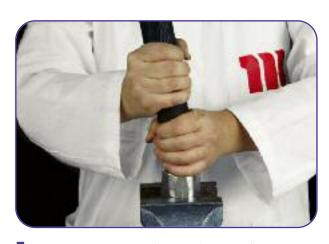
5 Secure in position the socket i.e. by using a benchvise.Screw the hose counterclockwise into the socket
